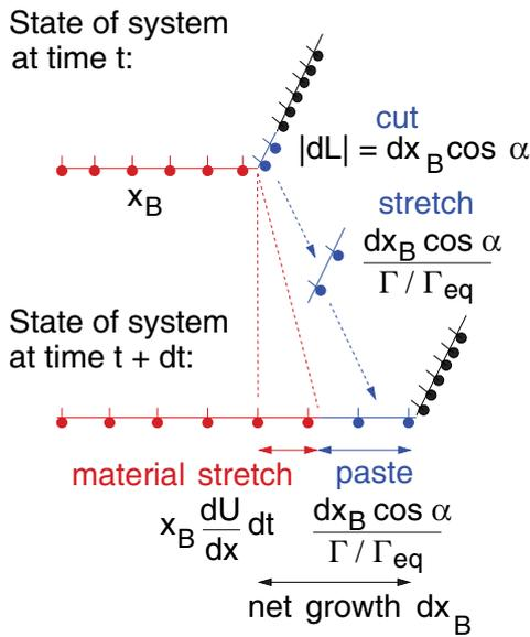
**Fig. 8.** The growth of  $x_B$  in the DS model viewed as a combination of a stretch operation (on the growing film) and a cut-stretch-paste operation (from the shrinking film to the growing film).
