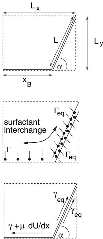
**Fig. 2.** Quadrant considered in the DS model. Upper figure: geometry of the quadrant; middle figure: surfactant interchange within the quadrant; lower figure: force balance on the quadrant.
