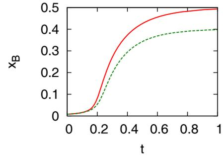
**Fig. 4.** Numerical solutions  $x_B$  vs.  $t$  for the DS model (all quantities are in dimensionless form). Upper curve is for  $\epsilon/\gamma_{\text{eq}} = 0$  and lower curve is for  $\epsilon/\gamma_{\text{eq}} = 1$ . The value  $x_0 = \frac{1}{128}$  was used here.
