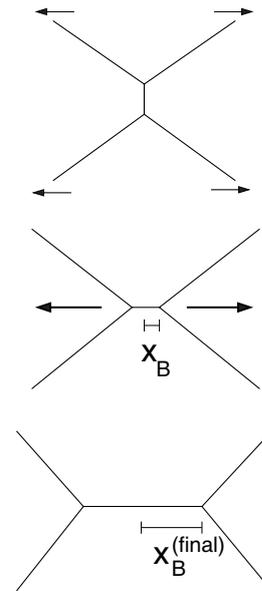
**Fig. 1.** Geometrical situation considered in the DS model: due to some imposed deformation (upper figure), a film disappears and is replaced (middle figure) by a reoriented, newly created film, which then grows over time towards a final equilibrium value (lower figure), whilst its neighbours shrink. The time evolution of the length  $2x_B$  of the growing film is of interest.
